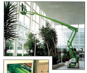
With more outreach than any other machine in its class and a base width of only 1.50m, the HR15N is one of the most effective and versatile self-propelled platforms available.
